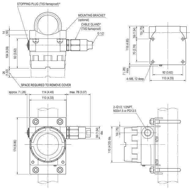
\*Two cable glands and one plug are provided with TIIS flameproof type. Use them according to the field wiring requirements.
